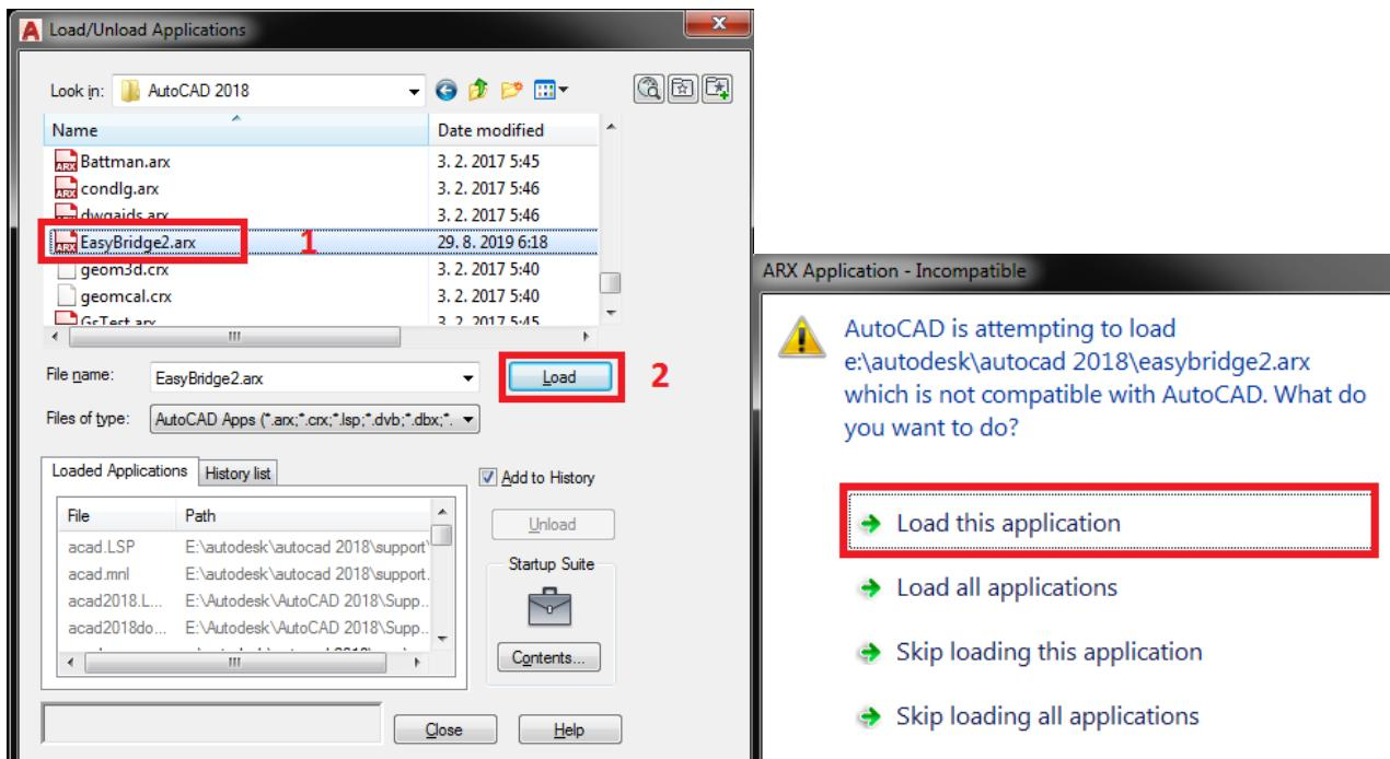
In installation folder of Easy Bridge find „EasyBridge2.arx“. Mark the file and with "Load" button load to AutoCAD. While loading, appears window with alert of incompatibility application with AutoCAD program. Confirm loading module. In this step program is loaded and you can run it with command "EasyBridge".
